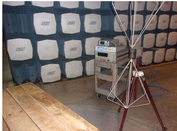
04 - System Check, Calibrated Signal @ 200 MHz
