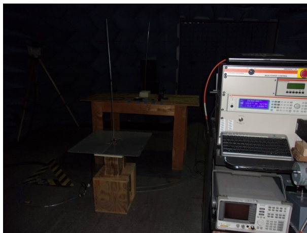
2 - 30MHz Radiated Stub
