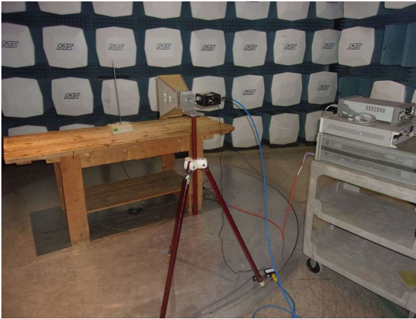
13 - System Check, Stub Radiator @ 18 GHz
