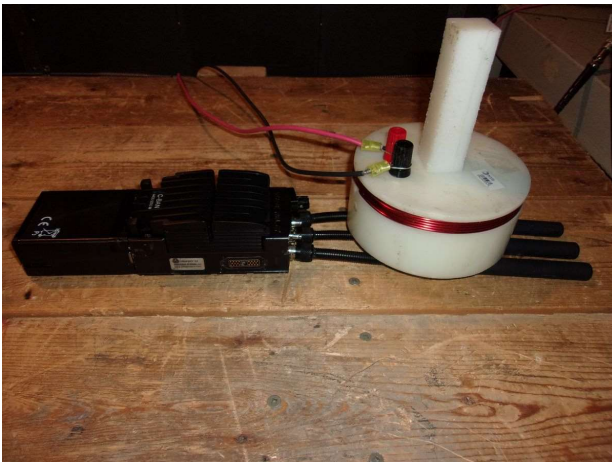
RS101 Test - Antennas
