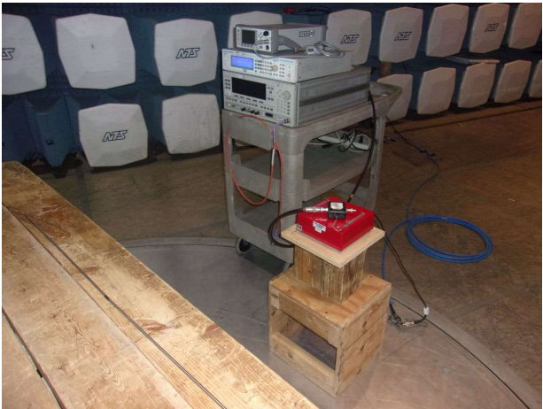
01 - System Check, Calibrated Signal 2 MHz - 30 MHz
