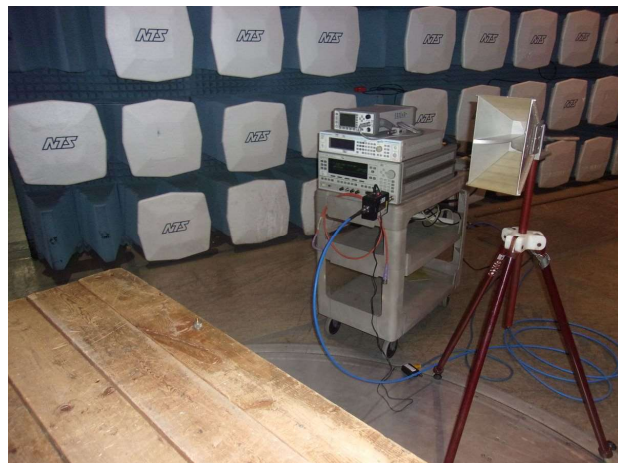
12 - System Check, Calibrated Signal @ 18 GHz
