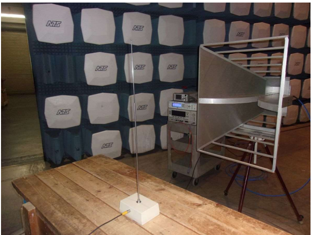
09 - System Check, Stub Radiator @ 1 GHz
